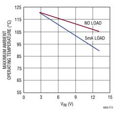
Figure 14. LTC6655-2.5 Maximum Ambient Operating Temperature
