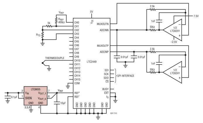
Low Noise Precision 24-Bit Analog-to-Digital Converter Application
