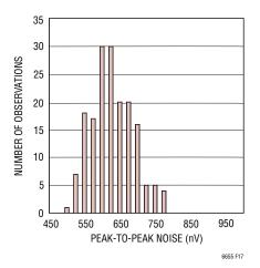
Figure 18. LTC6655-2.5 Low Frequency Noise Histogram
