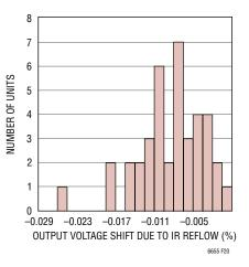
Figure 21. Output Voltage Shift Due to IR Reflow
