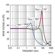
Figure 1. Output Voltage Noise Spectrum
