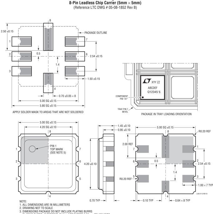
LS8 Package 8-Pin Leadless Chip Carrier ( $5mm \times 5mm$ )
