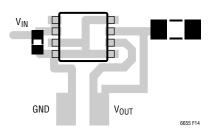
Figure 15. Sample PCB Layout
