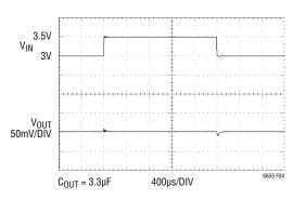
Figure 4. Output Response with a 500mV Step On  $\ensuremath{\text{V}_{\text{IN}}}$
