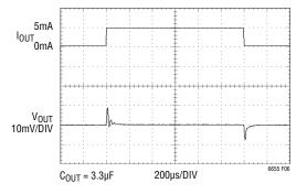
Figure 6. Output Response with 5mA Load Step Sinking
