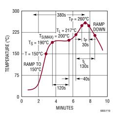
Figure 20. Lead-Free Reflow Profile
