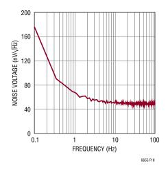
Figure 19. LTC6655-2.5 Low Frequency Noise Spectrum
