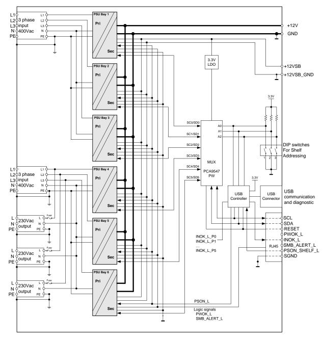
Figure 1. SPSPFE3-04G Block Diagram
