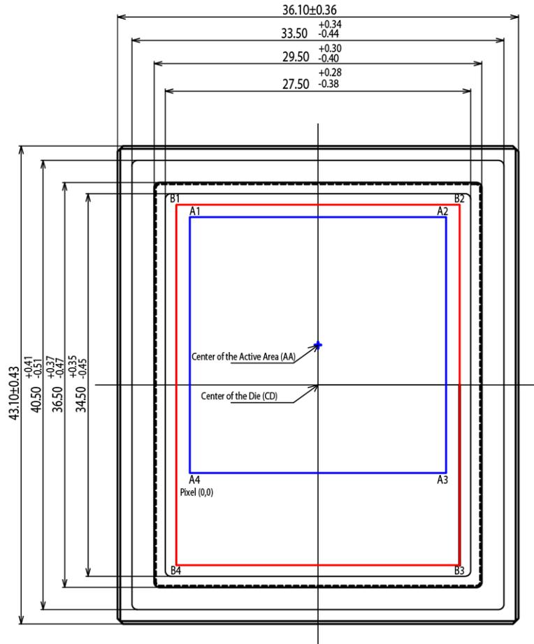
Figure 38. Graphical Representation of the Optical Center
