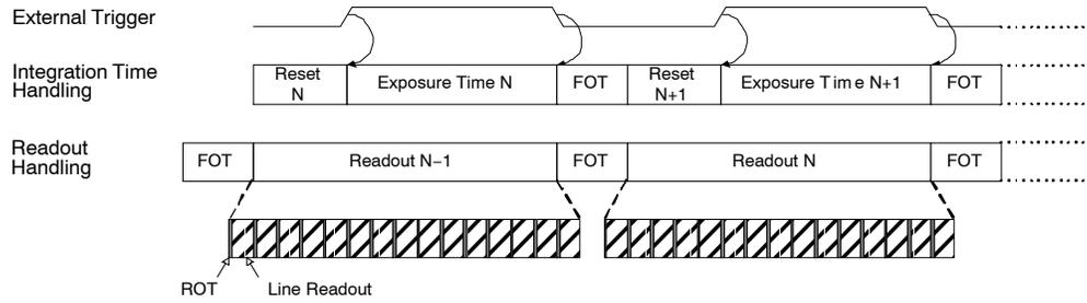
**Figure 9. Pipelined Shutter Operated in Slave Mode**
