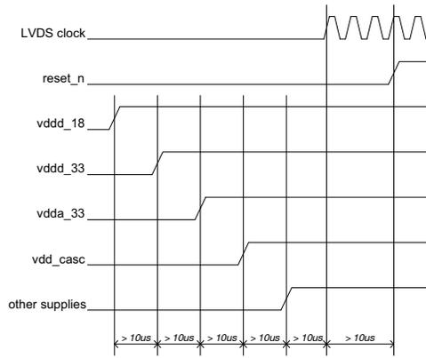
**Figure 13. Power-up Procedure**
