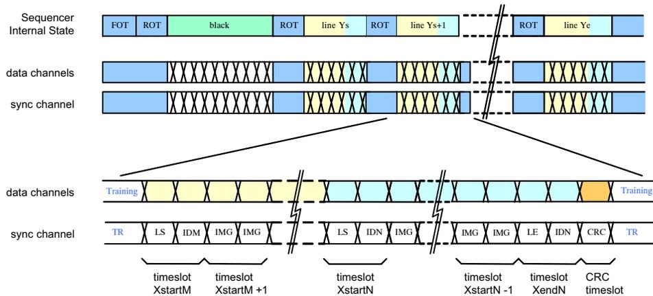
**Figure 30. Timeline Showing Readout of Two Overlapping Windows**
