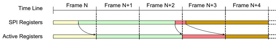
**Figure 15. Frame Synchronization of Configurations (no freezing)**
