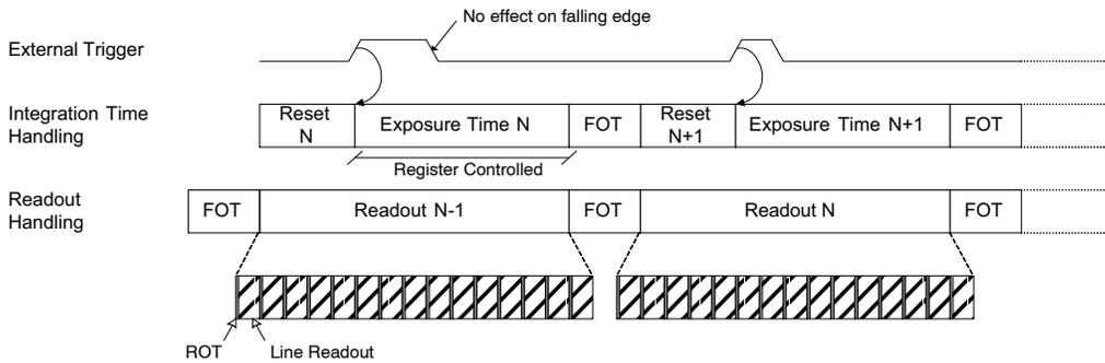
**Figure 10. Triggered Shutter Operated in Master Mode**
