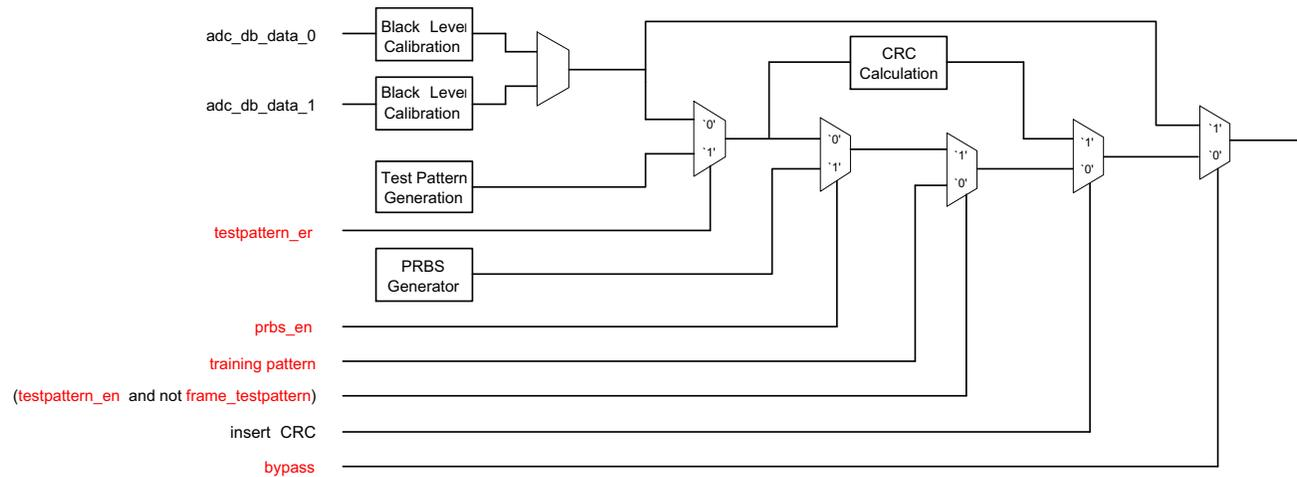
**Figure 36. Functional Block Diagrams for the Data Channels**
