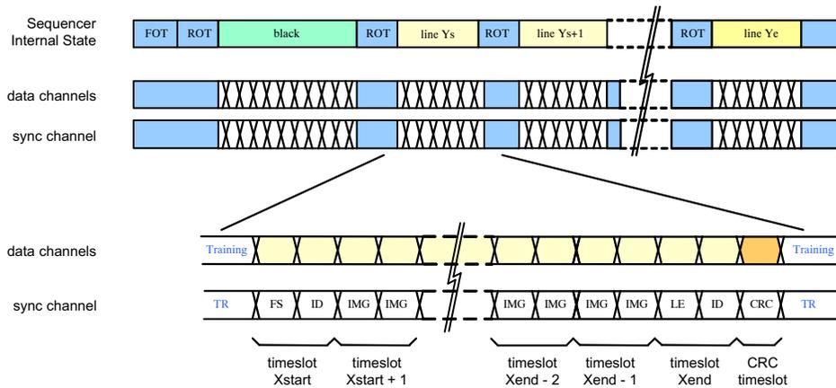
**Figure 29. Timeline for Single Window Readout**
