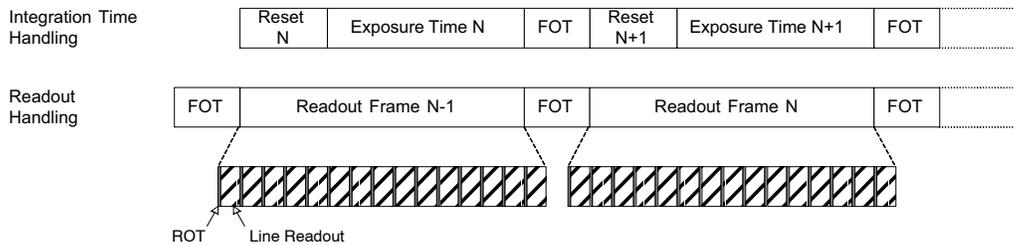
Figure 8. Integration and Readout for Pipelined Shutter
