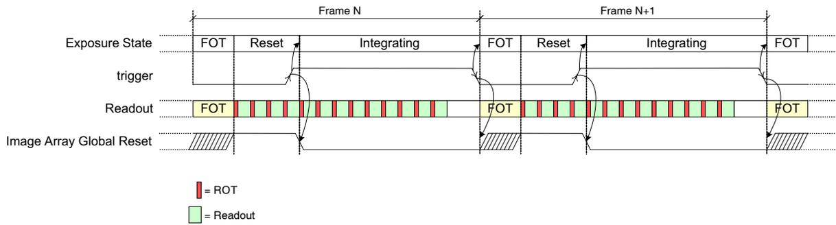
**Figure 21. Exposure Time Control in Global-Slave Mode**
