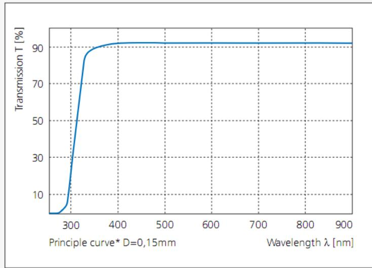
Figure 39. Transmission Characteristics of Glass Lid
