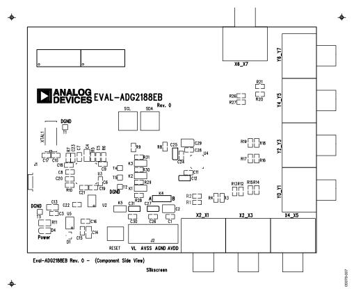
Figure 8. Component Placement Drawing
