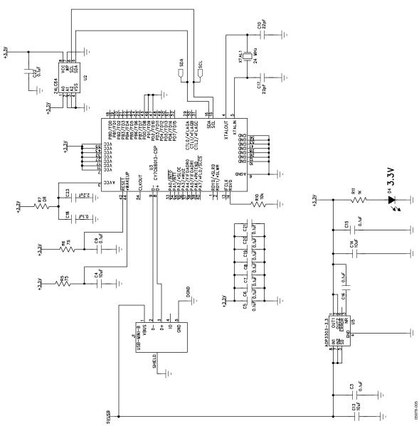
Figure 6. Schematic of USB Controller Circuitry
