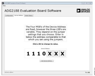
Figure 4. **Device Address** Tab
