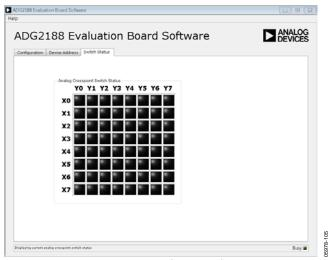
Figure 5. Switch Status Tab
