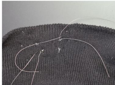
Next hook up the + connections from each of GEMMA's outputs to two pixels. We stitched from one sequin to the GEMMA, then over to another sequin and back to the first, making a sort of triangle that results in the thread tails being in the same place.
