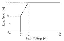
Fig.9.1 Input voltage derating curve (MGFS3, MGFW3, MGFS10, MGFW10)
