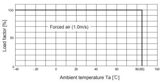
Fig.8.2 Derating Curve for Forced Air Cooling (1.0m/s) (Rated Input Voltage)
