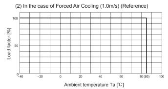
Fig.8.11 Derating Curve for Forced Air Cooling (1.0m/s) (Rated Input Voltage)
