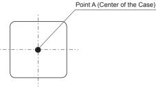
Fig.12.2 Temperature measuring point (Top View)
