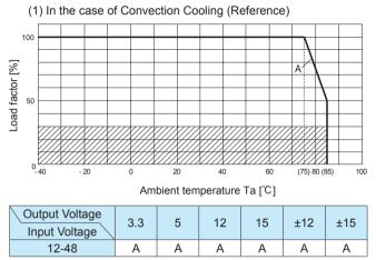
Fig.8.20 Derating Curve for Convection Cooling (Rated Input Voltage)
