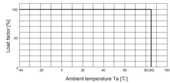
Fig.8.19 Derating Curve for Forced Air Cooling (1.0m/s) (Rated Input Voltage)
