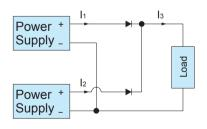
Fig.4.2 Redundancy operation
