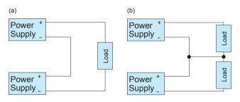
Fig.4.1 Examples of series operation
