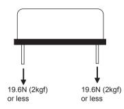
Fig.6.1 Stress onto Pins
