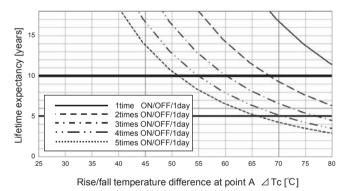
Fig.10.5 Lifetime expectancy against rise/fall temperature difference (MG10)
