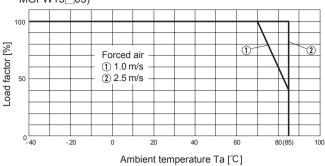
Fig.8.3 Derating Curve for Forced Air Cooling (1.0m/s,2.5m/s) (Rated Input Voltage)
