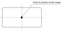
Fig.12.4 Temperature measuring point (Top View)
