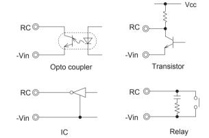
Fig.2.2 RC Connection Example
