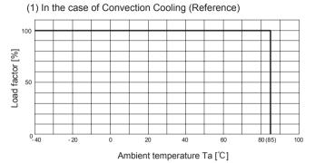
Fig.8.2 Derating Curve for Convection Cooling (Rated Input Voltage)
