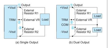
Fig.2.3 Connecting External Devices
