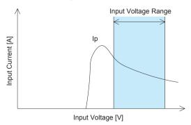
Fig.5.1 Input Current Characteristics
