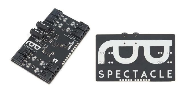
**Description:** The Spectacle Button Board allows you to add input from buttons, switches or other contact-type sensing devices to your Spectacle projects. This is the largest board in the Spectacle line due to its total of nine signal inputs, allowing for a large number of connections to a single module. Designed to bring simple signals from the world into your Spectacle projects, the Button Board provides input for any of your Spectacle projects!
