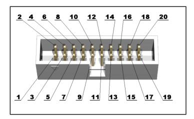
The JTAG connector allows the software debugger to talk via a JTAG (Joint Test Action Group) port directly to the core. Instructions may be inserted and executed by the core thus allowing STM32F107 memory to be programmed with code and executed step by step by the host software.
