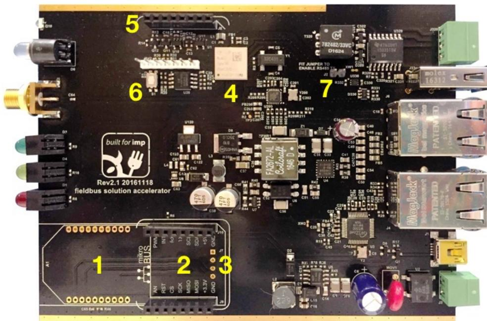
1. Header mounting pins for optional XBee module
