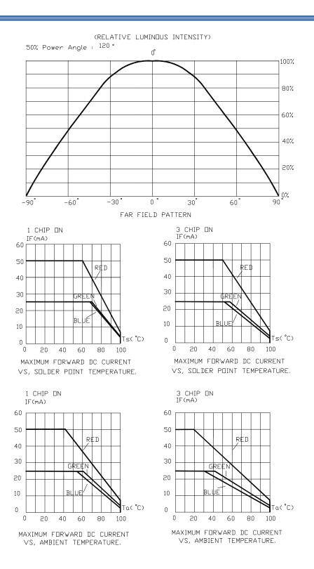
The above data are collected from statistical figures which do not necessarily correspond to the actual parameters of each single LED. Hence, these data will be changed without further notice.
