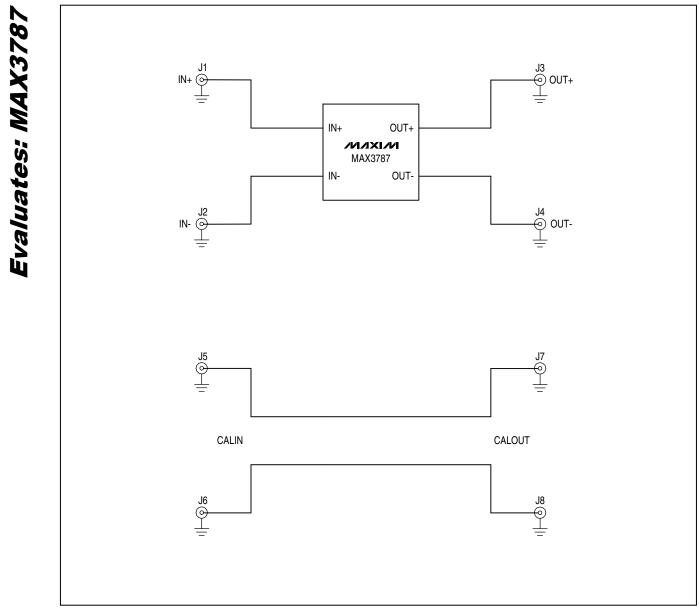
Figure 1. MAX3787 EV Kit Schematic
