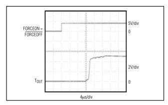
Figure 5. Transmitter Outputs Exiting Shutdown or Powering Up
