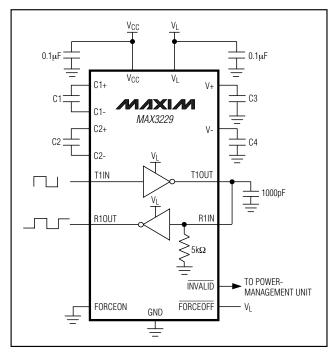
Figure 6. Transmitter Loopback Test Circuit
