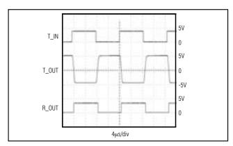
Figure 7. Loopback Test Result at 120kbps
