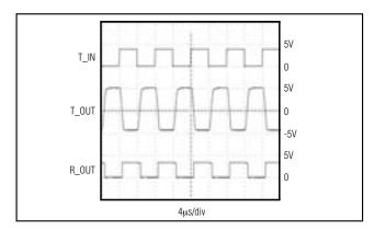
Figure 8. Loopback Test Result at 250kbps
