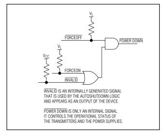
Figure 2c. MAX322\_ AutoShutdown Logic
