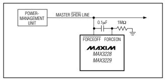
Figure 4. AutoShutdown with Initial Turn-On to Wake Up a System
