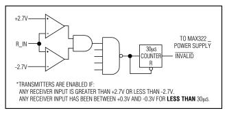
Figure 2b. MAX322\_ with Transmitters Enabled Using AutoShutdown
