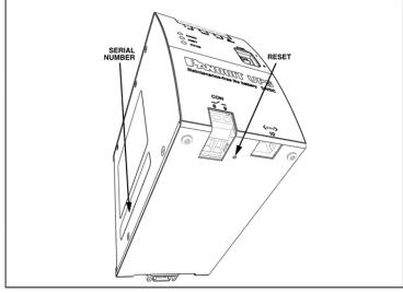
Figure 9: Reset Button Location
