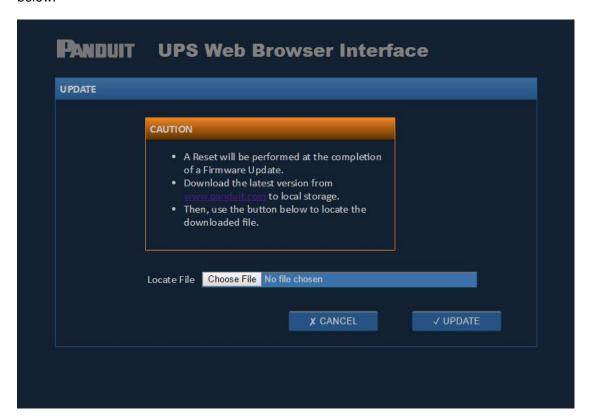
The image file should be downloaded and placed on an accessible network drive. After the image file is located and the UPDATE button is clicked, the UPS will import and update its software using the new image.
