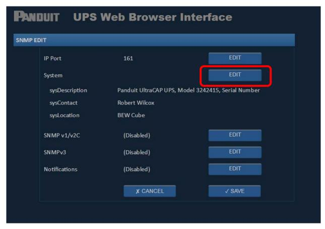
Enter a new name for the sysLocation and sysContact and press save. sysLocation and sysContact are used by network managers to indicate where the device is and who is responsible for managing it.
