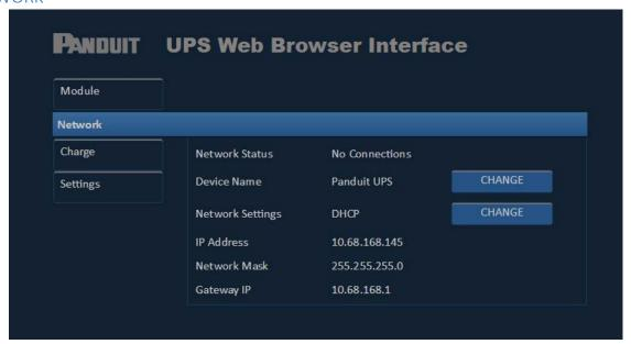
The network tab allows the Device Name and Network settings to be changed. For security, tab is Password protected. Use the network settings CHANGE button to set the DHCP or Static IP settings, IP Address, Network Mask, and Gateway IP.
