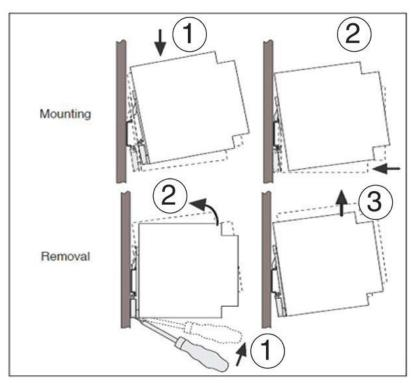
Figure 5: DIN Rail Installation
