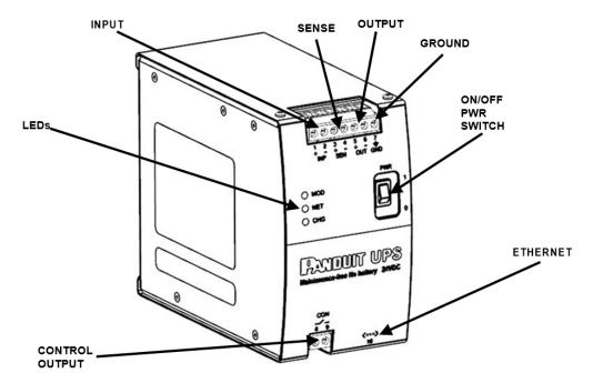
Figure 3: UPS Front Panel Details
