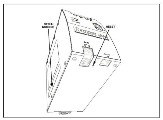
Figure 4: Reset Button and Serial Number
