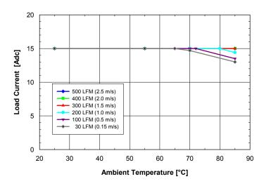
Fig. 2.0V.2: Available load current vs. ambient air temperature and airflow rates for **SQ24T15020** converter with **B** height pins mounted horizontally with Vin = 24V, air flowing from pin 3 to pin 1 and maximum FET temperature  $\leq 120^{\circ}$ C.
