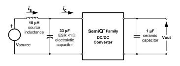
**Fig. 3.3V.14:** Test setup for measuring input reflected ripple currents,  $i_c$  and  $i_s$ .
