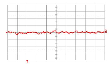
**Fig. 12V.16:** Input reflected ripple current,  $i_s$  (10 mA/div.), measured through 10 $\mu$ H at the source at full rated load current and Vin = 24V. Refer to Fig. 12V.14 for test setup. Time scale: 1 $\mu$ s/div.
