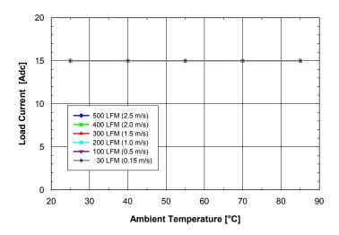
Fig. 1.5V.2: Available load current vs. ambient air temperature and airflow rates for **SQ24T15015** converter with **B** height pins mounted horizontally with Vin = 24V, air flowing from pin 3 to pin 1 and maximum FET temperature  $\leq 120^{\circ}$ C.
