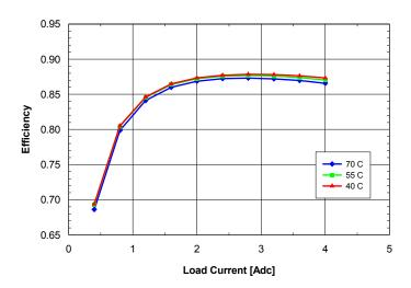
**Fig. 12V.6:** Efficiency vs. load current and ambient temperature for **SQ24T/S04120** converter mounted vertically with Vin = 24V and air flowing from pin 3 to pin 1 at a rate of 200 LFM (1.0 m/s).
