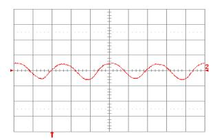
**Fig. 2.0V.15:** Input reflected ripple current,  $i_c$  (100 mA/div.), measured at input terminals at full rated load current and Vin = 24V. Refer to Fig. 2.0V.14 for test setup. Time scale: 1  $\mu$ s/div.
