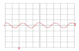
**Fig. 2.5V.15:** Input reflected ripple current,  $i_c$  (100 mA/div.), measured at input terminals at full rated load current and Vin = 24V. Refer to Fig. 2.5V.14 for test setup. Time scale: 1  $\mu$ s/div.
