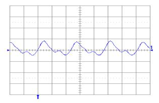
**Fig. 3.3V.13:** Output voltage ripple (20 mV/div.) at full rated load current into a resistive load with Co = 10  $\mu$ F tantalum + 1 $\mu$ F ceramic and Vin = 24 V. Time scale: 1  $\mu$ S/div.
