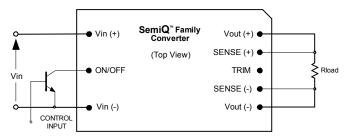
Fig. A: Circuit configuration for ON/OFF function.
