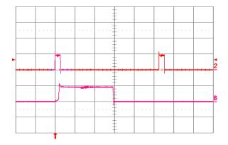
**Fig. 1.8V.18:** Load current (top trace, 20 A/div., 20 ms/div.) into a 10 m $\Omega$  short circuit during restart, at Vin = 24V. Bottom trace (20 A/div., 2 ms/div.) is an expansion of the on-time portion of the top trace.
