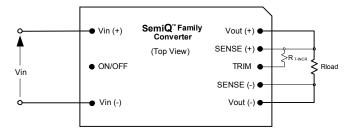
Fig. C: Configuration for increasing output voltage.
