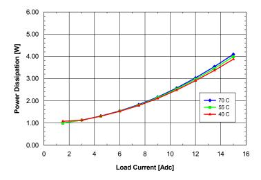
**Fig. 1.0V.8:** Power dissipation vs. load current and ambient temperature for **SQ24T/S15010** converter mounted vertically with Vin = 24V and air flowing from pin 3 to pin 1 at a rate of 200 LFM (1.0 m/s).
