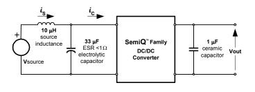
**Fig. 1.0V.14:** Test setup for measuring input reflected ripple currents,  $i_c$  and  $i_s$ .
