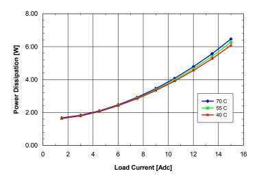
**Fig. 2.5V.8:** Power dissipation vs. load current and ambient temperature for **SQ24T/S15025** converter mounted vertically with Vin = 24V and air flowing from pin 3 to pin 1 at a rate of 200 LFM (1.0 m/s).
