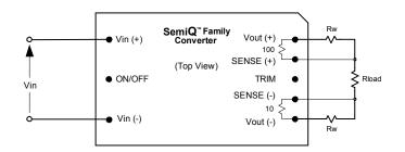
Fig. B: Remote sense circuit configuration.
