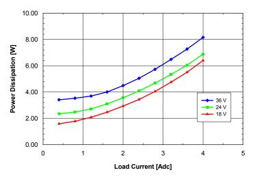
**Fig. 12V.7:** Power dissipation vs. load current and input voltage for **SQ24T/S04120** converter mounted vertically with air flowing from pin 3 to pin 1 at a rate of 300 LFM (1.5 m/s) and Ta = 25°C.
