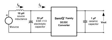
Fig. 1.8V.14: Test setup for measuring input reflected ripple currents,  $\dot{i}_c$  and  $\dot{i}_s$ .
