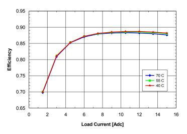
**Fig. 3.3V.6:** Efficiency vs. load current and ambient temperature for **SQ24T/S15033** converter mounted vertically with Vin = 24V and air flowing from pin 3 to pin 1 at a rate of 200 LFM (1.0 m/s).
