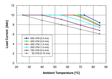
Fig. 5.0V.2: Available load current vs. ambient air temperature and airflow rates for **SQ24T10050** converter with **B** height pins mounted horizontally with Vin = 24V, air flowing from pin 3 to pin 1 and maximum FET temperature  $\leq 120^{\circ}$ C.
