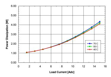
**Fig. 1.2V.8:** Power dissipation vs. load current and ambient temperature for **SQ24T/S15012** converter mounted vertically with Vin = 24V and air flowing from pin 3 to pin 1 at a rate of 200 LFM (1.0 m/s).
