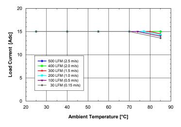
Fig. 1.8V.3: Available load current vs. ambient temperature and airflow rates for SQ24S15018 converter mounted vertically with Vin = 24V, air flowing from pin 3 to pin 1 and maximum FET temperature  $\leq$  120°C.
