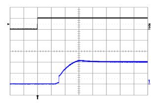
**Fig. 1.0V.10:** Turn-on transient at full rated load current (resistive) plus  $10,000\mu F$  at Vin = 24V, triggered via ON/OFF pin. Top trace: ON/OFF signal (5 V/div.). Bottom trace: output voltage (0.5 V/div.). Time scale: 1 ms/div.
