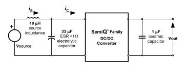
**Fig. 6.0V.14:** Test setup for measuring input reflected ripple currents,  $i_c$  and  $i_s$ .
