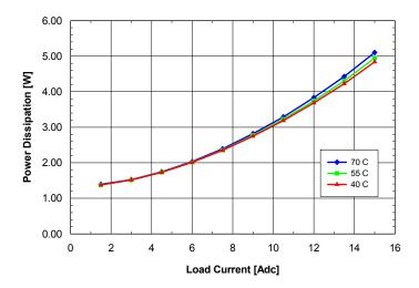
**Fig. 1.8V.8:** Power dissipation vs. load current and ambient temperature for **SQ24T/S15018** converter mounted vertically with Vin = 24V and air flowing from pin 3 to pin 1 at a rate of 200 LFM (1.0 m/s).
