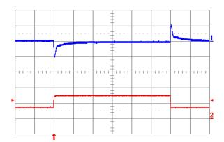
**Fig. 1.8V.12:** Output voltage response to load current stepchange (3.75A – 7.5A – 3.75A) at Vin = 24V. Top trace: output voltage (100 mV/div.). Bottom trace: load current (5 A/div.). Current slew rate: 5 A/μs. Co = 450 μF tantalum + 1 μF ceramic. Time scale: 0.2 ms/div.
