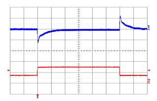
**Fig. 2.0V.12:** Output voltage response to load current stepchange (3.75A – 7.5A – 3.75A) at Vin = 24V. Top trace: output voltage (100 mV/div.). Bottom trace: load current (5 A/div.). Current slew rate: 5 A/μs. Co = 450 μF tantalum + 1 μF ceramic. Time scale: 0.2 ms/div.
