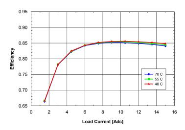
**Fig. 1.8V.6:** Efficiency vs. load current and ambient temperature for **SQ24T/S15018** converter mounted vertically with Vin = 24V and air flowing from pin 3 to pin 1 at a rate of 200 LFM (1.0 m/s).
