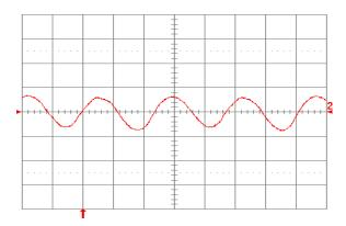
**Fig. 5.0V.15:** Input reflected ripple current,  $i_c$  (100 mA/div.), measured at input terminals at full rated load current and Vin = 24V. Refer to Fig. 5.0V.14 for test setup. Time scale: 1  $\mu$ s/div.
