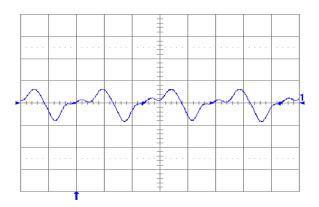
**Fig. 1.8V.13:** Output voltage ripple (20 mV/div.) at full rated load current into a resistive load with Co = 10  $\mu$ F tantalum + 1 $\mu$ F ceramic and Vin = 24 V. Time scale: 1  $\mu$ S/div.
