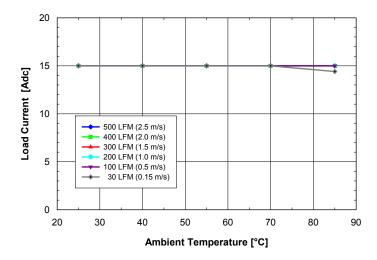
Fig. 1.8V.4: Available load current vs. ambient temperature and airflow rates for SQ24S15018 converter mounted horizontally with Vin = 24V, air flowing from pin 3 to pin 1 and maximum FET temperature  $\leq$  120°C.
