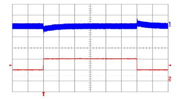
**Fig. 12V.11:** Output voltage response to load current step-change (1A - 2A - 1A) at Vin = 24V. Top trace: output voltage (200 mV/div.). Bottom trace: load current (1 A/div.). Current slew rate: 0.1 A/ $\mu$ s. Co = 1  $\mu$ F ceramic. Time scale: 0.5 ms/div.
