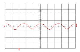
**Fig. 1.8V.15:** Input reflected ripple current,  $i_c$  (100 mA/div.), measured at input terminals at full rated load current and Vin = 24V. Refer to Fig. 1.8V.14 for test setup. Time scale: 1  $\mu$ s/div.
