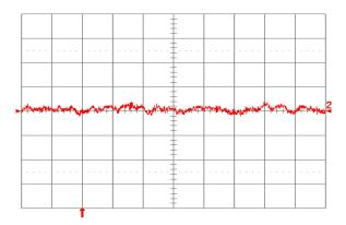
**Fig. 1.0V.16:** Input reflected ripple current,  $i_s$  (10 mA/div.), measured through 10  $\mu$ H at the source at full rated load current and Vin = 24V. Refer to Fig. 1.0V.14 for test setup. Time scale:  $1\mu s$ /div.
