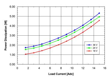
**Fig. 1.8V.7:** Power dissipation vs. load current and input voltage for **SQ24T/S15018** converter mounted vertically with air flowing from pin 3 to pin 1 at a rate of 300 LFM (1.5 m/s) and  $Ta = 25^{\circ}C$ .
