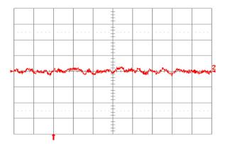
**Fig. 1.5V.16:** Input reflected ripple current,  $i_s$  (10 mA/div.), measured through 10  $\mu$ H at the source at full rated load current and Vin = 24V. Refer to Fig. 1.5V.14 for test setup. Time scale:  $1\mu$ s/div.
