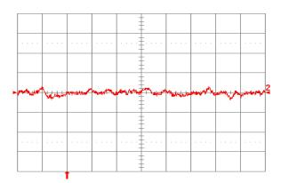
**Fig. 1.8V.16:** Input reflected ripple current,  $i_s$  (10 mA/div.), measured through 10  $\mu$ H at the source at full rated load current and Vin = 24V. Refer to Fig. 1.8V.14 for test setup. Time scale:  $1\mu$ s/div.
