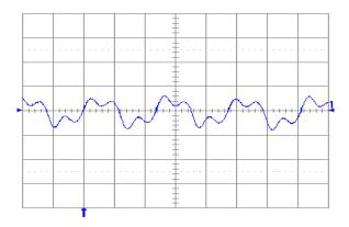
**Fig. 2.5V.13:** Output voltage ripple (20 mV/div.) at full rated load current into a resistive load with Co = 10  $\mu$ F tantalum + 1 $\mu$ F ceramic and Vin = 24 V. Time scale: 1  $\mu$ S/div.
