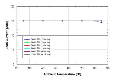
Fig. 1.8V.2: Available load current vs. ambient air temperature and airflow rates for **SQ24T15018** converter with **B** height pins mounted horizontally with Vin = 24V, air flowing from pin 3 to pin 1 and maximum FET temperature  $\leq 120^{\circ}$ C.
