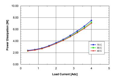
**Fig. 12V.8:** Power dissipation vs. load current and ambient temperature for **SQ24T/S04120** converter mounted vertically with Vin = 24V and air flowing from pin 3 to pin 1 at a rate of 200 LFM (1.0 m/s).
