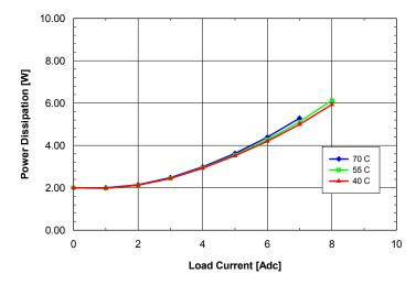
**Fig. 6.0V.8:** Power dissipation vs. load current and ambient temperature for **SQ24T/S08060** converter mounted vertically with Vin = 24V and air flowing from pin 3 to pin 1 at a rate of 200 LFM (1.0 m/s).
