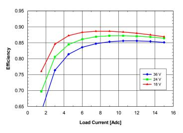
**Fig. 2.5V.5:** Efficiency vs. load current and input voltage for **SQ24T/S15025** converter mounted vertically with air flowing from pin 3 to pin 1 at a rate of 300 LFM (1.5 m/s) and  $Ta = 25^{\circ}C$ .
