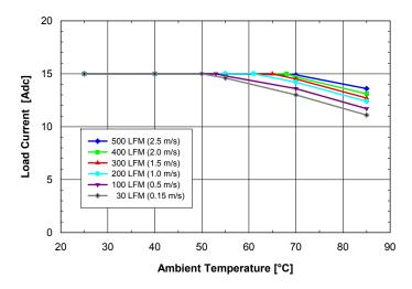
**Fig. 3.3V.4:** Available load current vs. ambient temperature and airflow rates for **SQ24S15033** converter mounted horizontally with Vin = 24V, air flowing from pin 3 to pin 1 and maximum FET temperature  $\leq$  120°C.
