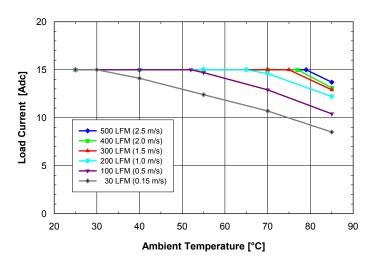
Fig. 3.3V.2: Available load current vs. ambient air temperature and airflow rates for **SQ24T15033** converter with **B** height pins mounted horizontally with Vin = 24V, air flowing from pin 3 to pin 1 and maximum FET temperature  $\leq 120^{\circ}$ C.
