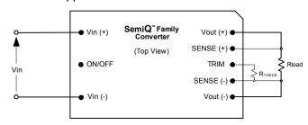
Fig. D: Configuration for decreasing output voltage.
