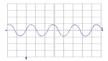
**Fig. 12V.13:** Output voltage ripple (50 mV/div.) at full rated load current into a resistive load with Co = 10  $\mu$ F tantalum + 1 $\mu$ F ceramic and Vin = 24 V. Time scale: 1  $\mu$ S/div.
