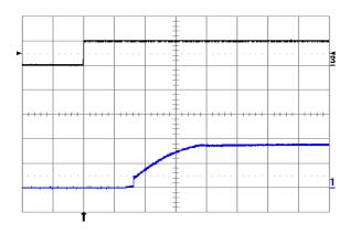
**Fig. 1.8V.10:** Turn-on transient at full rated load current (resistive) plus  $10,000\mu F$  at Vin = 24V, triggered via ON/OFF pin. Top trace: ON/OFF signal (5 V/div.). Bottom trace: output voltage (1 V/div.). Time scale: 1 ms/div.
