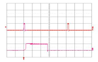
**Fig. 3.3V.18:** Load current (top trace, 20 A/div., 20 ms/div.) into a 10 m $\Omega$  short circuit during restart, at Vin = 24V. Bottom trace (20 A/div., 1 ms/div.) is an expansion of the on-time portion of the top trace.
