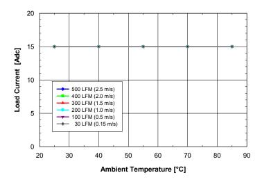
Fig. 1.2V.2: Available load current vs. ambient air temperature and airflow rates for **SQ24T15012** converter with **B** height pins mounted horizontally with Vin = 24V, air flowing from pin 3 to pin 1 and maximum FET temperature  $\leq 120^{\circ}$ C.
