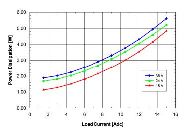
**Fig. 2.0V.7:** Power dissipation vs. load current and input voltage for **SQ24T/S15020** converter mounted vertically with air flowing from pin 3 to pin 1 at a rate of 300 LFM (1.5 m/s) and  $Ta = 25^{\circ}C$ .
