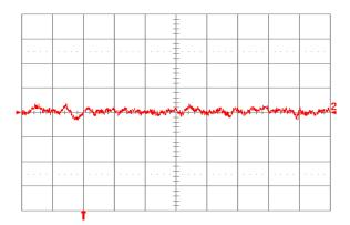
**Fig. 2.5V.16:** Input reflected ripple current,  $i_s$  (10 mA/div.), measured through 10  $\mu$ H at the source at full rated load current and Vin = 24V. Refer to Fig. 2.5V.14 for test setup. Time scale:  $1\mu s$ /div.
