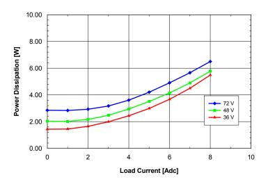
**Fig. 6.0V.7:** Power dissipation vs. load current and ambient temperature for **SQ24T/S08060** converter mounted vertically with air flowing from pin 3 to pin 1 at a rate of 300 LFM (1.5 m/s) and  $Ta = 25^{\circ}C$ .
