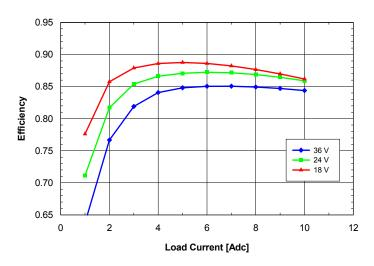
**Fig. 5.0V.5:** Efficiency vs. load current and input voltage for **SQ24T/S10050** converter mounted vertically with air flowing from pin 3 to pin 1 at a rate of 300 LFM (1.5 m/s) and  $Ta = 25^{\circ}C$ .
