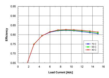
**Fig. 1.2V.6:** Efficiency vs. load current and ambient temperature for **SQ24T/S15012** converter mounted vertically with Vin = 24V and air flowing from pin 3 to pin 1 at a rate of 200 LFM (1.0 m/s).
