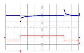
**Fig. 1.0V.12:** Output voltage response to load current stepchange (3.75 A - 7.5 A - 3.75 A) at Vin = 24V. Top trace: output voltage (100 mV/div.). Bottom trace: load current (5 A/div.). Current slew rate: 5 A/ $\mu$ s. Co = 450 μF tantalum + 1 μF ceramic. Time scale: 0.2 ms/div.
