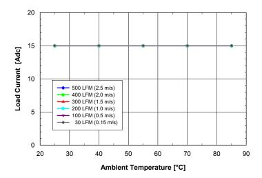
**Fig. 1.2V.4:** Available load current vs. ambient temperature and airflow rates for **SQ24S15012** converter mounted horizontally with Vin = 24V, air flowing from pin 3 to pin 1 and maximum FET temperature  $\leq$  120°C.
