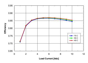
**Fig. 5.0V.6:** Efficiency vs. load current and ambient temperature for **SQ24T/S10050** converter mounted vertically with Vin = 24V and air flowing from pin 3 to pin 1 at a rate of 200 LFM (1.0 m/s).
