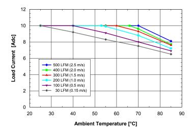
**Fig. 5.0V.4:** Available load current vs. ambient temperature and airflow rates for **SQ24S10050** converter mounted horizontally with Vin = 24V, air flowing from pin 3 to pin 1 and maximum FET temperature  $\leq$  120°C.
