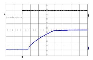
**Fig. 6.0V.10:** Turn-on transient at full rated load current (resistive) plus  $10,000\mu\text{F}$  at Vin = 24V, triggered via ON/OFF pin. Top trace: ON/OFF signal (5 V/div.). Bottom trace: output voltage (2 V/div.). Time scale: 2 ms/div.
