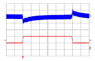
**Fig. 6.0V.11:** Output voltage response to load current step-change (2A-4A-2A) at Vin = 24V. Top trace: output voltage (100mV/div.). Bottom trace: load current (2A/div.). Current slew rate: 0.1 A/ $\mu$ s. Co = 1  $\mu$ F ceramic. Time scale: 0.2 ms/div.
