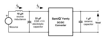
Fig. 5.0V.14: Test setup for measuring input reflected ripple currents,  $\dot{\textbf{i}}_c$  and  $\dot{\textbf{i}}_s$ .
