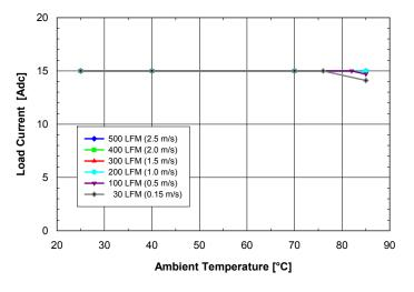
Fig. 1.5V.3: Available load current vs. ambient temperature and airflow rates for SQ24S15015 converter mounted vertically with Vin = 24V, air flowing from pin 3 to pin 1 and maximum FET temperature  $\leq$  120°C.
