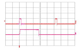
**Fig. 1.5V.18:** Load current (top trace, 20 A/div., 20 ms/div.) into a 10 m $\Omega$  short circuit during restart, at Vin = 24V. Bottom trace (20 A/div., 2 ms/div.) is an expansion of the on-time portion of the top trace.
