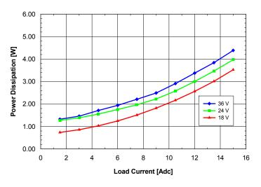
**Fig. 1.0V.7:** Power dissipation vs. load current and input voltage for **SQ24T/S15010** converter mounted vertically with air flowing from pin 3 to pin 1 at a rate of 300 LFM (1.5 m/s) and  $Ta = 25^{\circ}C$ .
