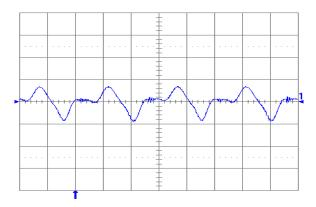
**Fig. 1.5V.13:** Output voltage ripple (20 mV/div.) at full rated load current into a resistive load with Co = 10  $\mu$ F tantalum + 1 $\mu$ F ceramic and Vin = 24 V. Time scale: 1  $\mu$ S/div.
