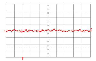
**Fig. 1.2V.16:** Input reflected ripple current,  $i_s$  (10 mA/div.), measured through 10  $\mu$ H at the source at full rated load current and Vin = 24V. Refer to Fig. 1.2V.14 for test setup. Time scale:  $1\mu$ s/div.
