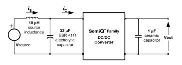
**Fig. 1.5V.14:** Test setup for measuring input reflected ripple currents,  $i_c$  and  $i_s$ .
