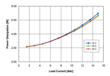
**Fig. 3.3V.8:** Power dissipation vs. load current and ambient temperature for **SQ24T/S15033** converter mounted vertically with Vin = 24V and air flowing from pin 3 to pin 1 at a rate of 200 LFM (1.0 m/s).
