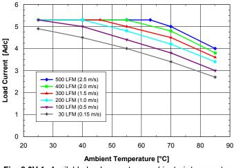
Fig. 8.0V.1: Available load current vs. ambient air temperature and airflow rates for **SQ24T05080** converter with **D** height pins mounted vertically with Vin = 24 V, air flowing from pin 3 to pin 1 and maximum FET temperature  $\leq 120^{\circ}$ C.
