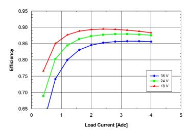
**Fig. 12V.5:** Efficiency vs. load current and input voltage for **SQ24T/S04120** converter mounted vertically with air flowing from pin 3 to pin 1 at a rate of 300 LFM (1.5 m/s) and Ta = 25°C.
