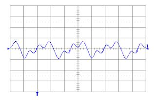
**Fig. 2.0V.13:** Output voltage ripple (20 mV/div.) at full rated load current into a resistive load with Co = 10  $\mu$ F tantalum + 1 $\mu$ F ceramic and Vin = 24 V. Time scale: 1  $\mu$ S/div.
