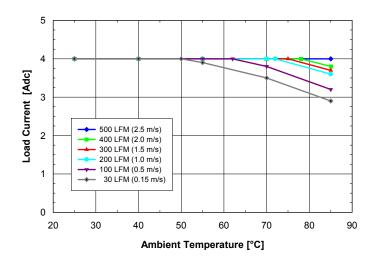
**Fig. 12V.4:** Available load current vs. ambient temperature and airflow rates for **SQ24S04120** converter mounted horizontally with Vin = 24V, air flowing from pin 3 to pin 1 and maximum FET temperature  $\leq$  120°C.
