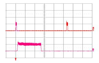
**Fig. 12V.18:** Load current (top trace, 5 A/div., 20 ms/div.) into a 10 m $\Omega$  short circuit during restart, at Vin = 24V. Bottom trace (5 A/div., 1 ms/div.) is an expansion of the on-time portion of the top trace.
