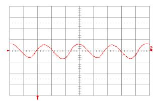
**Fig. 6.0V.15:** Input reflected ripple current,  $i_c$  (100 mA/div.), measured at input terminals at full rated load current and Vin = 24V. Refer to Fig. 6.0V.14 for test setup. Time scale: 1  $\mu$ s/div.
