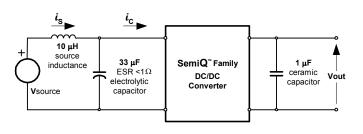
**Fig. 2.0V.14:** Test setup for measuring input reflected ripple currents,  $i_c$  and  $i_s$ .
