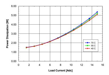
**Fig. 2.0V.8:** Power dissipation vs. load current and ambient temperature for **SQ24T/S15020** converter mounted vertically with Vin = 24V and air flowing from pin 3 to pin 1 at a rate of 200 LFM (1.0 m/s).
