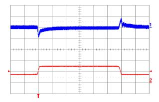
**Fig. 1.8V.11:** Output voltage response to load current stepchange (3.75A - 7.5A - 3.75A) at Vin = 24V. Top trace: output voltage (100 mV/div.). Bottom trace: load current (5 A/div.). Current slew rate: 0.1 A/ $\mu$ s. Co = 1  $\mu$ F ceramic. Time scale: 0.2 ms/div.
