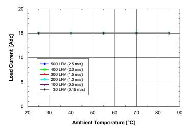
Fig. 1.2V.3: Available load current vs. ambient temperature and airflow rates for SQ24S15012 converter mounted vertically with Vin = 24V, air flowing from pin 3 to pin 1 and maximum FET temperature  $\leq$  120°C.
