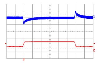
**Fig. 1.0V.11:** Output voltage response to load current stepchange (3.75 A - 7.5 A - 3.75 A) at Vin = 24V. Top trace: output voltage (100 mV/div.). Bottom trace: load current (5 A/div.). Current slew rate: 0.1 A/ $\mu$ s. Co = 1  $\mu$ F ceramic. Time scale: 0.2 ms/div.
