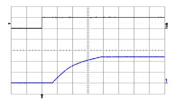
**Fig. 12V.10:** Turn-on transient at full rated load current (resistive) plus  $1{,}000\mu\text{F}$  at Vin = 24V, triggered via ON/OFF pin. Top trace: ON/OFF signal (5 V/div.). Bottom trace: output voltage (5 V/div.). Time scale: 2 ms/div.
