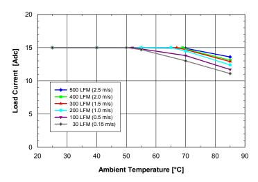
**Fig. 2.5V.4:** Available load current vs. ambient temperature and airflow rates for **SQ24S15025** converter mounted horizontally with Vin = 24V, air flowing from pin 3 to pin 1 and maximum FET temperature  $\leq$  120°C.
