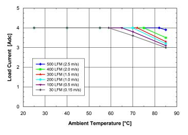
**Fig. 12V.3:** Available load current vs. ambient temperature and airflow rates for **SQ24S04120** converter mounted vertically with Vin = 24V, air flowing from pin 3 to pin 1 and maximum FET temperature  $\leq$  120°C.
