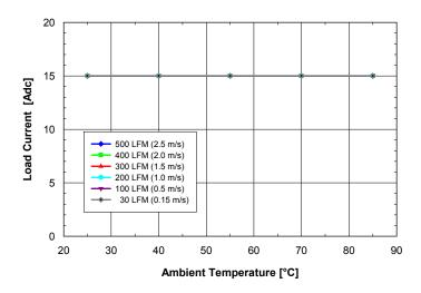
Fig. 1.0V.2: Available load current vs. ambient air temperature and airflow rates for **SQ24T15010** converter with **B** height pins mounted horizontally with Vin = 24V, air flowing from pin 3 to pin 1 and maximum FET temperature  $\leq 120^{\circ}$ C.
