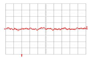
**Fig. 5.0V.16:** Input reflected ripple current,  $i_s$  (10 mA/div.), measured through 10  $\mu$ H at the source at full rated load current and Vin = 24V. Refer to Fig. 5.0V.14 for test setup. Time scale:  $1\mu$ s/div.
