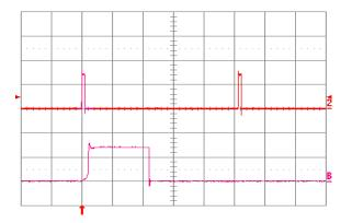
**Fig. 5.0V.18:** Load current (top trace, 10 A/div., 20 ms/div.) into a 10 m $\Omega$  short circuit during restart, at Vin = 24V. Bottom trace (10 A/div., 1 ms/div.) is an expansion of the on-time portion of the top trace.
