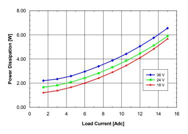
**Fig. 2.5V.7:** Power dissipation vs. load current and input voltage for **SQ24T/S15025** converter mounted vertically with air flowing from pin 3 to pin 1 at a rate of 300 LFM (1.5 m/s) and  $Ta = 25^{\circ}C$ .
