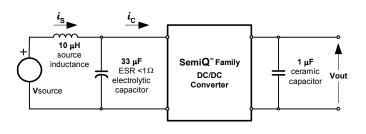
**Fig. 12V.14:** Test setup for measuring input reflected ripple currents,  $i_c$  and  $i_s$ .
