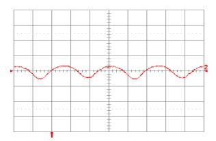
**Fig. 1.2V.15:** Input reflected ripple current,  $i_c$  (100 mA/div.), measured at input terminals at full rated load current and Vin = 24V. Refer to Fig. 1.2V.14 for test setup. Time scale: 1  $\mu$ s/div.
