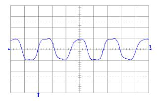
**Fig. 5.0V.13:** Output voltage ripple (20 mV/div.) at full rated load current into a resistive load with Co = 10  $\mu$ F tantalum + 1 $\mu$ F ceramic and Vin = 24 V. Time scale: 1  $\mu$ S/div.
