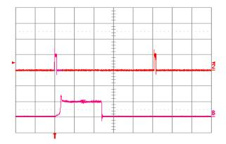
**Fig. 2.5V.18:** Load current (top trace, 20 A/div., 20 ms/div.) into a 10 m $\Omega$  short circuit during restart, at Vin = 24V. Bottom trace (20 A/div., 1 ms/div.) is an expansion of the on-time portion of the top trace.
