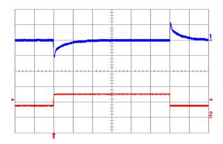
**Fig. 2.5V.12:** Output voltage response to load current stepchange (3.75 A - 7.5 A - 3.75 A) at Vin = 24V. Top trace: output voltage (100 mV/div.). Bottom trace: load current (5 A/div.). Current slew rate: 5 A/μs. Co = 450 μF tantalum + 1 μF ceramic. Time scale: 0.2 ms/div.
