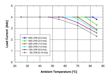
**Fig. 12V.1:** Available load current vs. ambient air temperature and airflow rates for **SQ24T04120** converter with **B** height pins mounted vertically with Vin = 24V, air flowing from pin 3 to pin 1 and maximum FET temperature ≤ 120°C.
