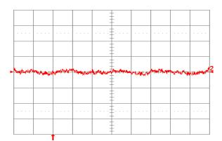
**Fig. 6.0V.16:** Input reflected ripple current,  $i_s$  (10 mA/div.), measured through 10  $\mu$ H at the source at full rated load current and Vin = 24V. Refer to Fig. 6.0V.14 for test setup. Time scale:  $1\mu$ S/div.
