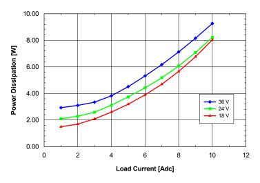
**Fig. 5.0V.7:** Power dissipation vs. load current and input voltage for **SQ24T/S10050** converter mounted vertically with air flowing from pin 3 to pin 1 at a rate of 300 LFM (1.5 m/s) and Ta = 25°C.
