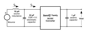
**Fig. 2.5V.14:** Test setup for measuring input reflected ripple currents,  $i_c$  and  $i_s$ .
