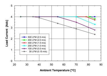
**Fig. 12V.2:** Available load current vs. ambient air temperature and airflow rates for **SQ24T04120** converter with **B** height pins mounted horizontally with Vin = 24V, air flowing from pin 3 to pin 1 and maximum FET temperature  $\leq$  120°C.
