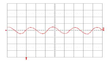
**Fig. 12V.15:** Input reflected ripple current,  $i_c$  (100 mA/div.), measured at input terminals at full rated load current and Vin = 24V. Refer to Fig. 12V.14 for test setup. Time scale: 1  $\mu$ s/div.
