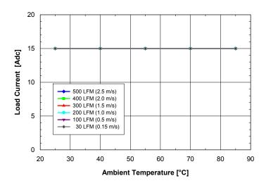
**Fig. 1.5V.4:** Available load current vs. ambient temperature and airflow rates for **SQ24S15015** converter mounted horizontally with Vin = 24V, air flowing from pin 3 to pin 1 and maximum FET temperature  $\leq$  120°C.
