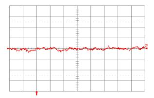
**Fig. 3.3V.16:** Input reflected ripple current,  $i_s$  (10 mA/div.), measured through 10  $\mu$ H at the source at full rated load current and Vin = 24V. Refer to Fig. 3.3V.14 for test setup. Time scale:  $1\mu$ s/div.
