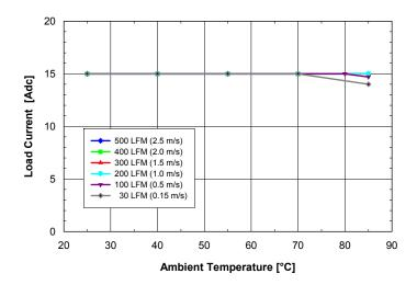
**Fig. 2.0V.4:** Available load current vs. ambient temperature and airflow rates for **SQ24S15020** converter mounted horizontally with Vin = 24V, air flowing from pin 3 to pin 1 and maximum FET temperature  $\leq$  120°C.
