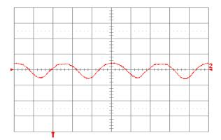
**Fig. 1.5V.15:** Input reflected ripple current,  $i_c$  (100 mA/div.), measured at input terminals at full rated load current and Vin = 24V. Refer to Fig. 1.5V.14 for test setup. Time scale: 1  $\mu$ s/div.
