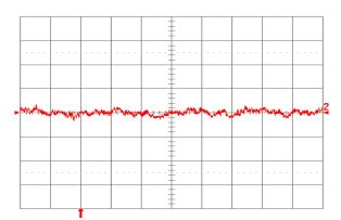
**Fig. 2.0V.16:** Input reflected ripple current,  $i_s$  (10 mA/div.), measured through 10  $\mu$ H at the source at full rated load current and Vin = 24V. Refer to Fig. 2.0V.14 for test setup. Time scale:  $1\mu$ S/div.
