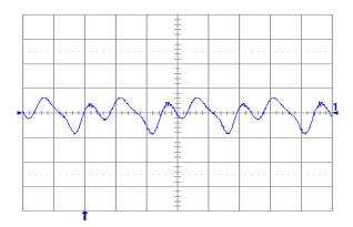
**Fig. 1.2V.13:** Output voltage ripple (20 mV/div.) at full rated load current into a resistive load with Co = 10  $\mu$ F tantalum + 1 $\mu$ F ceramic and Vin = 24 V. Time scale: 1  $\mu$ S/div.
