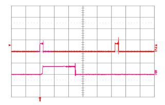
**Fig. 6.0V.18:** Load current (top trace, 20 A/div., 20 ms/div.) into a 10 m $\Omega$  short circuit during restart, at Vin = 24V. Bottom trace (20 A/div., 2 ms/div.) is an expansion of the on-time portion of the top trace.
