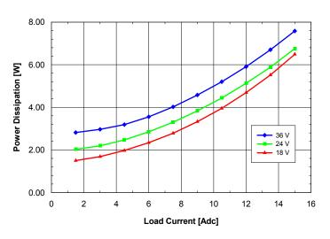
**Fig. 3.3V.7:** Power dissipation vs. load current and input voltage for **SQ24T/S15033** converter mounted vertically with air flowing from pin 3 to pin 1 at a rate of 300 LFM (1.5 m/s) and Ta = 25°C.
