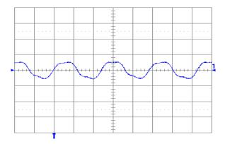
**Fig. 6.0V.13:** Output voltage ripple (50 mV/div.) at full rated load current into a resistive load with Co = 10  $\mu$ F tantalum + 1 $\mu$ F ceramic and Vin = 24 V. Time scale: 1  $\mu$ S/div.
