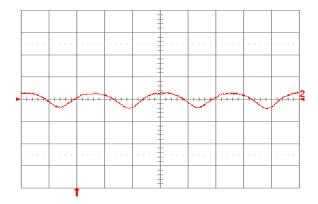
**Fig. 1.0V.15:** Input reflected ripple current,  $i_c$  (100 mA/div.), measured at input terminals at full rated load current and Vin = 24V. Refer to Fig. 1.0V.14 for test setup. Time scale: 1  $\mu$ s/div.
