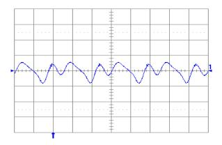
**Fig. 1.0V.13:** Output voltage ripple (20 mV/div.) at full rated load current into a resistive load with Co = 10  $\mu$ F tantalum + 1 $\mu$ F ceramic and Vin = 24 V. Time scale: 1  $\mu$ S/div.
