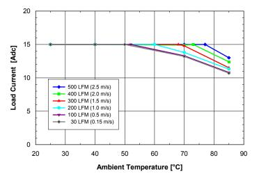
Fig. 3.3V.3: Available load current vs. ambient temperature and airflow rates for SQ24S15033 converter mounted vertically with Vin = 24V, air flowing from pin 3 to pin 1 and maximum FET temperature  $\leq$  120°C.
