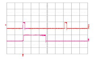
**Fig. 2.0V.18:** Load current (top trace, 20 A/div., 20 ms/div.) into a 10 m $\Omega$  short circuit during restart, at Vin = 24V. Bottom trace (20 A/div., 2 ms/div.) is an expansion of the on-time portion of the top trace.
