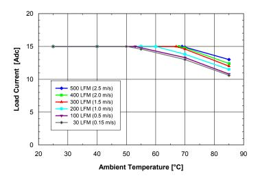
**Fig. 2.5V.3:** Available load current vs. ambient temperature and airflow rates for **SQ24S15025** converter mounted vertically with Vin = 24V, air flowing from pin 3 to pin 1 and maximum FET temperature  $\leq$  120°C.
