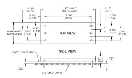
**SQ24T Pinout (Through-hole)**
