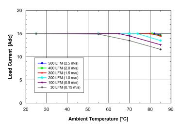
Fig. 2.5V.2: Available load current vs. ambient air temperature and airflow rates for SQ24T15025 converter with B height pins mounted horizontally with Vin = 24V, air flowing from pin 3 to pin 1 and maximum FET temperature  $\leq$  120°C.
