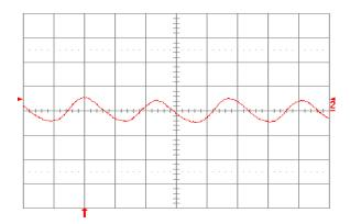
**Fig. 3.3V.15:** Input reflected ripple current,  $i_c$  (100 mA/div.), measured at input terminals at full rated load current and Vin = 24V. Refer to Fig. 3.3V.14 for test setup. Time scale: 1  $\mu$ s/div.
