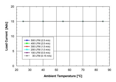
**Fig. 1.0V.1:** Available load current vs. ambient air temperature and airflow rates for **SQ24T15010** converter with **B** height pins mounted vertically with Vin = 24V, air flowing from pin 3 to pin 1 and maximum FET temperature  $\leq 120^{\circ}$ C.
